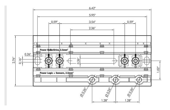
To be able to position the magnetic key, the distance from the top edge of MultiControl to adjacent components must be at least 0.4".
