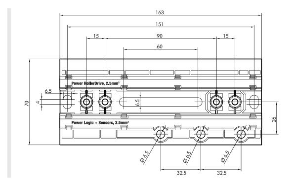
To be able to position the magnetic key, the distance from the top edge of MultiControl to adjacent components must be at least 10 mm.
