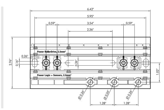
To be able to position the magnetic key, the distance from the top edge of MultiControl to adjacent components must be at least 0.4".
